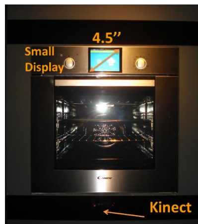
Fig. 4. Front view of MOTIC with the integrated small display and Kinect sensing device
